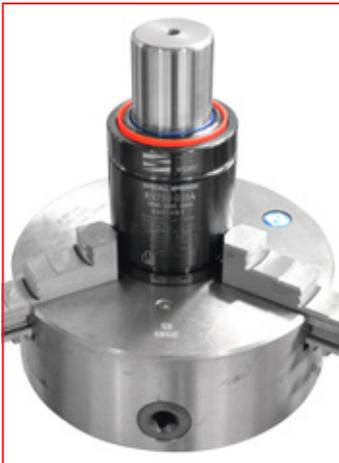
1- Secure the cylinder onto a self-centring chuck or a vice.
