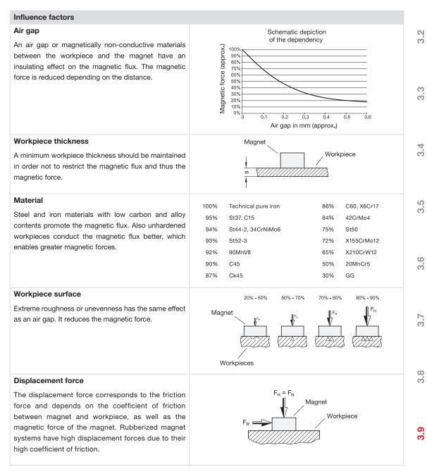
The nominal magnetic forces stated in the tables on the series pages are minimum values obtained at room temperature, vertical "tear-off" and full-surface contact of the magnet with low carbon steel workpieces and a minimum thickness of 10 mm.
