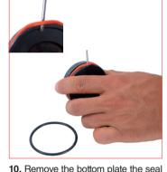
without scratching the internal groove.
