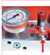
A. After positioning and hosing all the cylinders, proceed through the quick fit device trough the control panel for charging all the cylinders. 39DMCPVA control panel charging
