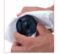
tom plate. If the bottom plate show any wear or damage do not use it again and replace it with a new one.
