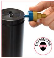
2. Thread DDS discharging device on the charging port then exhaust completely the pressure. Point away from the operator for maximum safety. **39DDS01A** BLUE side for M6 hole GOLD side for 1/8"G hole
