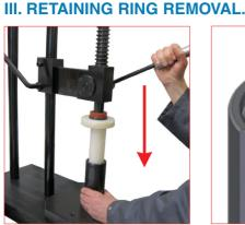
5. Position the anti scratch nylon removal tube (49TN...) on the bottom plate then by the manual press (39PM02A) press all down into the body. The retaining ring is now free for an easy removal.
