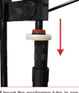
22.Insert the positioning tube in contact with the retaining C-ring, then by the manual press, press down the retaining C-ring into the groove. When the C-ring enter correctly into the groove you will hear a loud like "CLICK". 49TB... conical centring guide tube.
