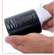
11. Carefully check and clean the 12. Carefully check and clean the 13. Carefully check and clean the botcylinder body. If the body show any wear or damage do not use it again and replace it with a new one.
