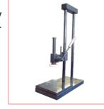
Cod. 49TB079 (ML12000B) Reassembly guiding tube for the bushing + reassembly positioning tube for the retaining C-ring.
