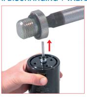
1. Remove the protective screw cap from the charging hole by using the appropriate tool Preserve the the protective screw cap for further reassembly **58CE05** for the 1/8 G port.
