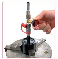
30. When directly charging throught the adapter and desired pressure is reached shut off the hose and bottle valves and disconnect the the quick fit coupling.
