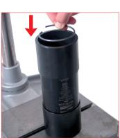
21. Position the retaining C-ring into the conical centring guide tube.
