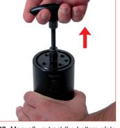
23. Manually extract the bottom plate untill it rests against the C-ring. 58EM06 T handle M6 58EM08+58EM1/8G T handle 1/8"G
