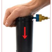
3. Be sure the pressure is completley exhauted by pressing down the piston rod into the cylinder body. Then unthread the discharging device from the discharging hole.
