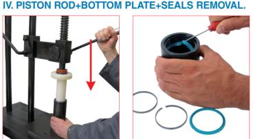
9. Remove from the cylinder body all the seals and guiding elements without scratching the internal groo-
