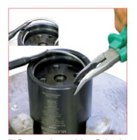
7. Remove the retaining C-ring by using the appropriate removal tool Preserve the retaining C-ring for further reassembly. 58EAR C-ring removal tool.
