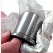
piston-rod. If the piston-rod shows any damage, wear or scratch do not use it again
