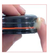
17. Lubrificate all the installed components into the bottom plate with the Special Springs grease.
