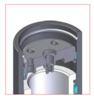
**5.1.** Cut off of cylinder to see the right position of the bottom plate and C-ring after operation.
