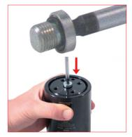
**34.** It is always recommended to **35.** Thread the protective screw into the charging hole by using the appropriate tool. 58CE05 for 1/8G charging port. 58CE03 for M6 charging port.
