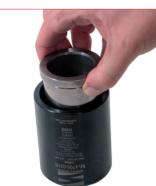
18. Manually insert the piston rod into the cylinder body. Be care to position it on the correct side.
