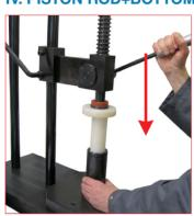
8. With the manual press (39PM02A) and with he anti scratch nylon tube (49TN..), press down the piston rod into the cylinder body in order to remove it completely.
