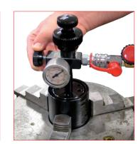
29. Rached and stabilized the desired pressure, for an easy and safety work carefully follow the instructions supplied with the charging unit. **39DMA** charging unit.
