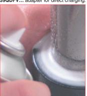
check leaks on the upper side of the cylinders after the maintenance work and before re-using the cylinders by using the special gas detector. 39RFG Special Springs gas detector.
