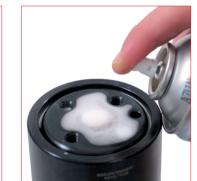
33. It is always recommended to check leaks on the charging port after the maintenance work and before re-using the cylinders by using the special gas detector.
