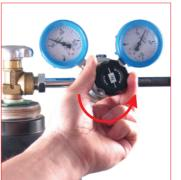
27. Adjust the required maximum pressure trought the regulation valve. The gauge on the right will indicate the maximum allowed pressure to charge the cylinder. 39R... pressure regulation valve.
