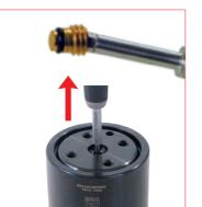
4. Hang and release the one way valve from the hole by using the appropriate tool. It would be normal some oil leak from the hole when upside down the cylinder. 58CD01 one way valve removingsetting dynamometric wrench.
