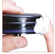
24. Lubrificate all the installed elements using the Special Spring grease.
