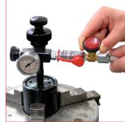
charging adapter and thread it on the charging port. For an easy and safe operation carefully follow the instructions supplied with the charging unit. DO NOT exceed the maximum pressure indicated for any specific model. 39DMA charging unit.
