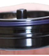
18. Assembly the dual ring on the bottom base as shown on the picture. Pav attention NOT to twist the dual-ring.
