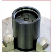
7. Position and clamp the cylinder into a self - centring chuck or a vice.
