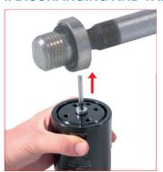
1. Remove the protective plug from the charging hole by using the appropriate tool. Preserve the protective plug for further reassembly. 58CE05 for the 1/8 G port. 58CE03 for the M6 port.
