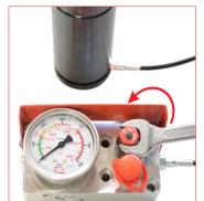
A. To exhaust pressure of linked cilynders open the discharging valve on the control panel.
