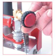
C. Connect the female quick fit on the male quick fit on the panel and open the gas tap. For an easy and safe operation carefully follow the instructions supplied with the charging unit. 39DMCPVA control panel charging
