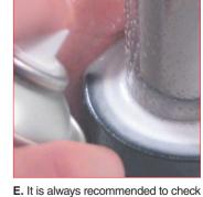
leaks on the upper side of the cylinders after the maintenance work and before re-using the cylinders by using the special gas detector. 39RFG Special Springs gas detector.
