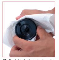
17. Carefully check and clean the bottom base, blowing inside pressurized air to remove residuals from the dual-ring groove and charging port. If the bottom base shows any wear or damage DO NOT use it again and replace it with a new one.
