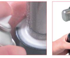
41. It is always recommended to check leaks on the upper side of the cylinders after the maintenance work and before re-using the cylinders by using the special gas detector. 39RFG Special Springs gas detector
