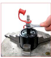
**38.** Unthread and release the adapter from the charging hole.
