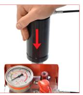
B. Be sure the pressure is completley exhausted by pressing down the piston rod into the cilynders body.
