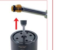
4. Unscrew and remove the one way valve from the hole by using the appropriate tool. It would be normal some oil leak from the hole when upside down the cylinder. **58CD01** Torque wrench for one way
