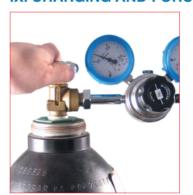
33. Check the correct assembly of 34. Adjust the required maximum 35. Select and assemble the desired 36. Once reached and stabilized the the pressure regulation valve on the gas bottle, then open the main tap. The gauge on the left will indicate the
