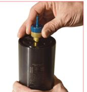
2. Thread DDS discharging device on the charging port then exhaust completely the pressure. Point away from the operator for maximum safety. 39DDS01A BLUE side for M6 hole GOLD side for 1/8"G hole
