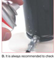
leaks on all connections to and from the cylinder by using the special gas detector 39RFG Special Springs gas detector.
