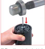
**42.** Thread the protective plug into the charging hole by using the appropri-**58CE05** for 1/8G charging port.
