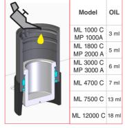
28. Put inside the cylinder the lubricating oil in the correct quantity as mentioned above **5900LIO** Special Springs Oil
