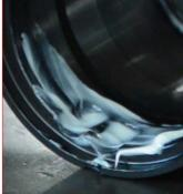
25. Lubricate the bottom grooves using the Special Springs grease. **590GRASSO** Special Springs grease
