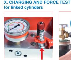
A. After positioning and hosing all the cylinders, proceed through the quick fit device in the control panel for charging all the cylinders. 39DMCPVA control panel charging unit.
