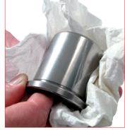
16. Carefully check and clean the rod. If the rod shows any damage, wear or scratch DO NOT use it again and replace it with a new one
